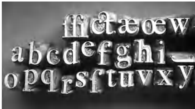
Actual Bodoni "type." Carved punches were driven into other pieces of metal called matrices. Molten metal was then poured into these matrices, making the actual type. Courtesy of Sumner Stone.
